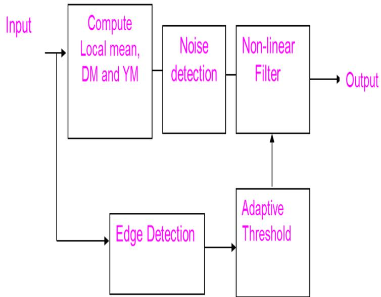
Fig 2: Block diagram of noise detection using adaptive filter
